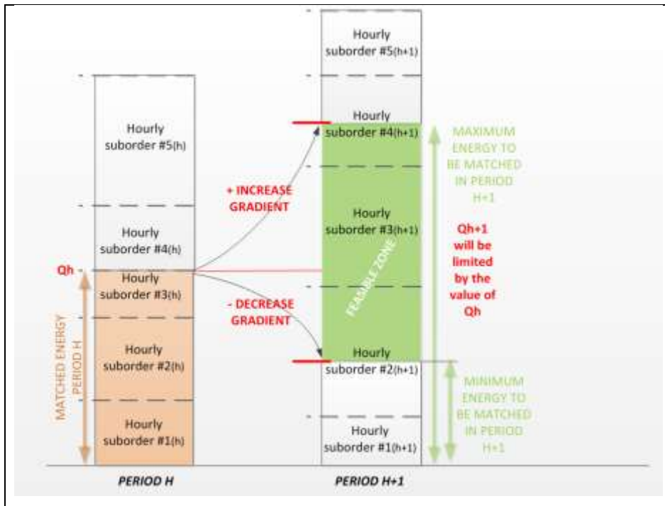
Figure 9 – A Load Gradient order. Effect produced by the amount that is matched in period (h) on period (h+1).
